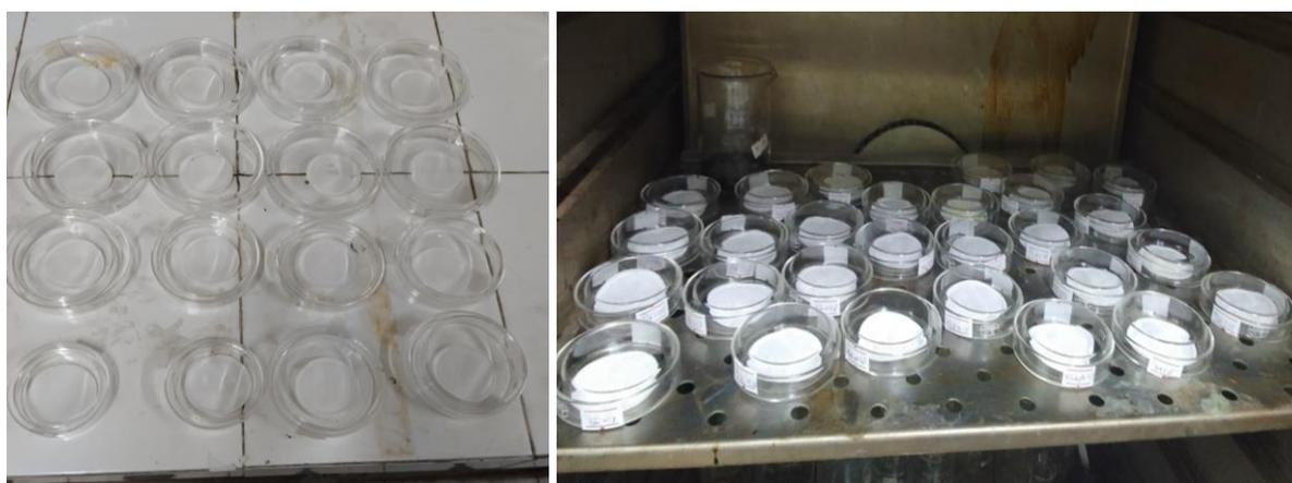
**Fig. 30.** Filters before (left) and after (right) the filtration process.
