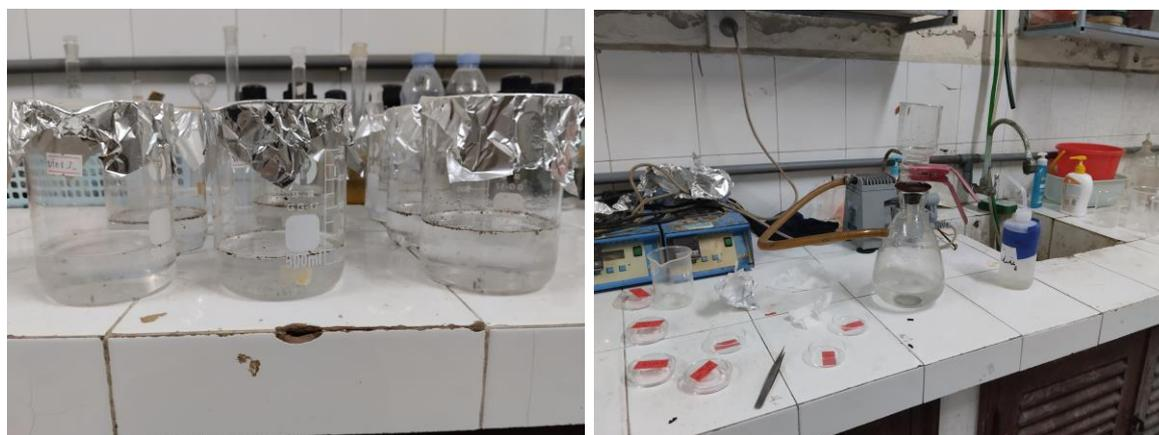
**Fig. 27.** Organic material digestion (left) and filtration to collect floating fragments (right)
