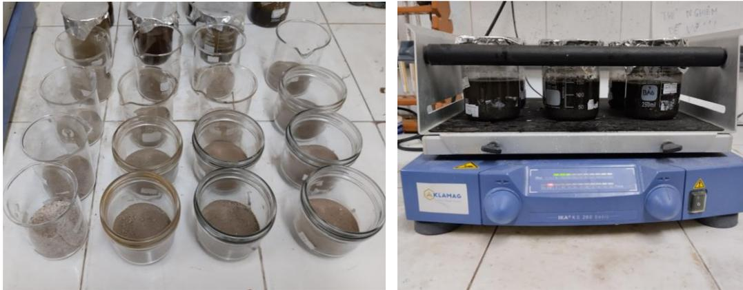
**Fig. 28.** Dried sediment (left) and shaking process on a shaker (right)
