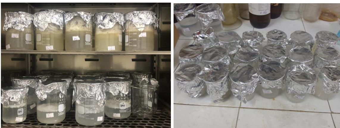
**Fig. 29.** GIT dissolution (left) and density separation process (right).
