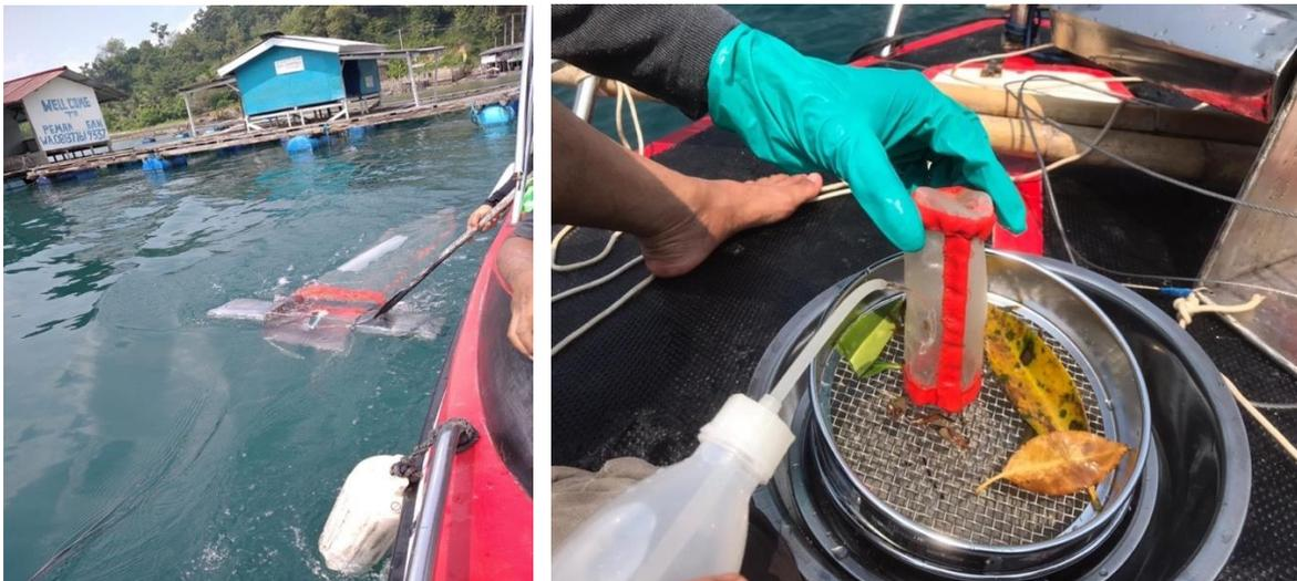
**Fig. 7.** Surface water sampling around net cages by a Manta net.
