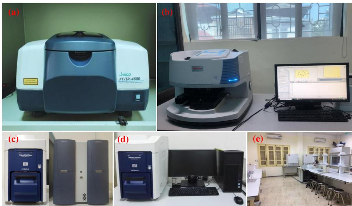
**Fig. 32.** FT – IR Spectroscopy JASCO 4600 (a),  $\mu$  FT – IR NICOLET iN10, Thermo Scientific, USA (b), Scanning Electron Microscopy (SEM) coupled with Energy-dispersive X-ray spectroscopy (EDX) (c), and preparation room (d)
